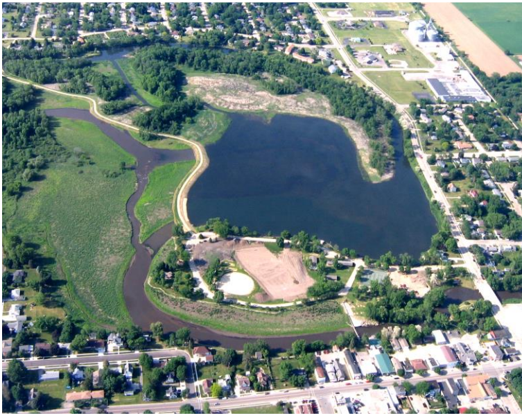
Figure 3. Diversion of the Sugar River around Lake Belle View.
